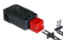
Safety microswitch with separated actuator, with release electromagnet – to pull out the actuator when the coil is energized – 24 VAC-DC coil – no. 2 NC contacts – complete with straight and bent key.
