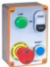
Four-operators pushbutton panel, with Start-Stop pushbutton (no. 1 NC + no. 1 NO contact) + led warning light 12/30 V ac-dc, emergency mushroom-shaped pushbutton (no. 1 NC contact), green warning light, blue reset button (no. 1 NC contact), IP65
