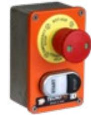
Two-operators pushbutton panel, with Start-Stop-Warning Light pushbutton, led warning-light 12/30 V ac-dc, (nr. 1 NC + nr. 1 NO contact) – emergency mushroom-shaped pushbutton (nr. 1 NC contact) – Yellow label Ø 60 “Emergency”, IP65
