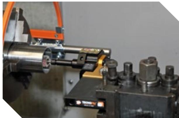
Grinding the inner surface.
