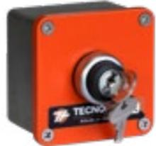
Single operator pushbutton panel, with two stable positions selector 0 – 1 and removable key, nr. 1 NC contact, IP65
