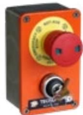
Two-operators pushbutton panel, with two stable positions selector 0 – 1 and removable key, (no. 1 NC contact) – emergency mushroom-shaped pushbutton (no. 1 NC contact) – Yellow label Ø 60 “Emergency”, IP65
