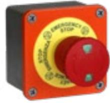
Single operator pushbutton panel, with emergency mushroom-shaped pushbutton (nr. 1 NC contact) – Yellow label Ø 60 “Emergency”, IP65
